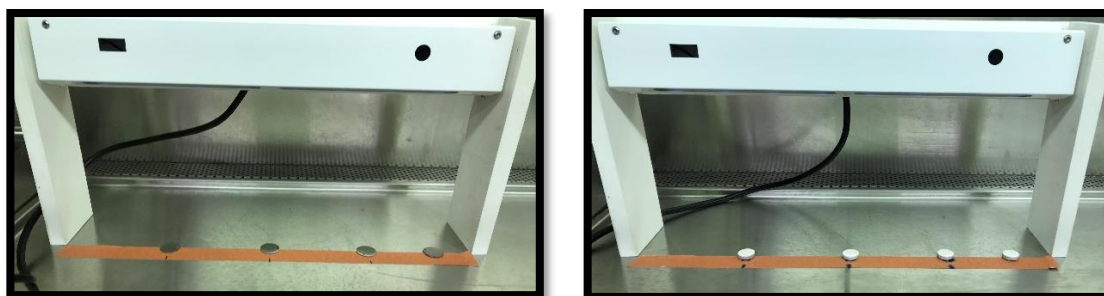
Figure 3: SteriLumen® SLR-1 Disinfecting Bar with Test Samples (stainless steel coupon (left) and ceramic coupon (right))
