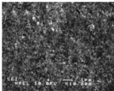
g) E. coli on a microscope slide coated with catalyst, exposed to UV light (254 nm) for 75 hours.
